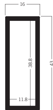
Z 100 Beam extrusion 43 mm 3.14 kg | 5000 mm
